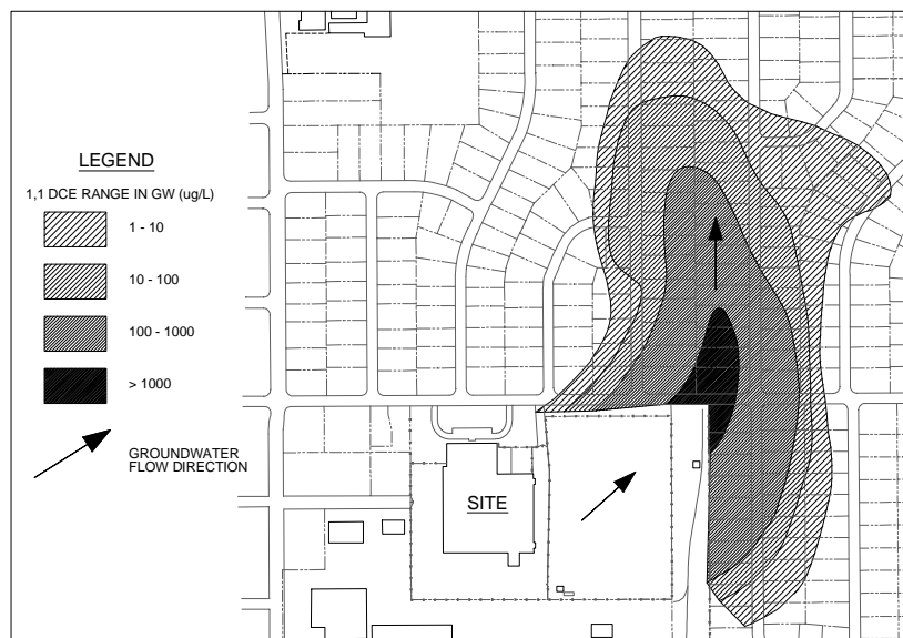
Figure 1. 1,1 DCE plume in groundwater.
