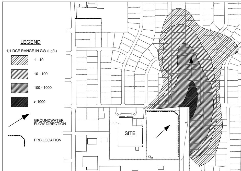
Figure 2. 1,1 DCE plume in groundwater.
