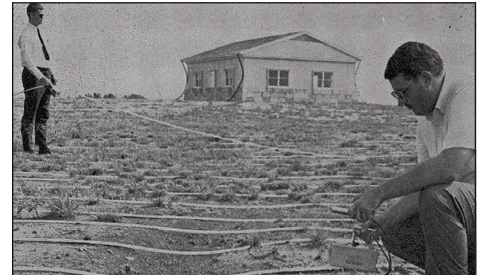
Nuclear engineering faculty are conducting tests of simulated nuclear fallout under a $99,567 research contract for the DOD on a "typical American house." The house is part of K-State's million-dollar 180-acre test site five miles west of campus.
