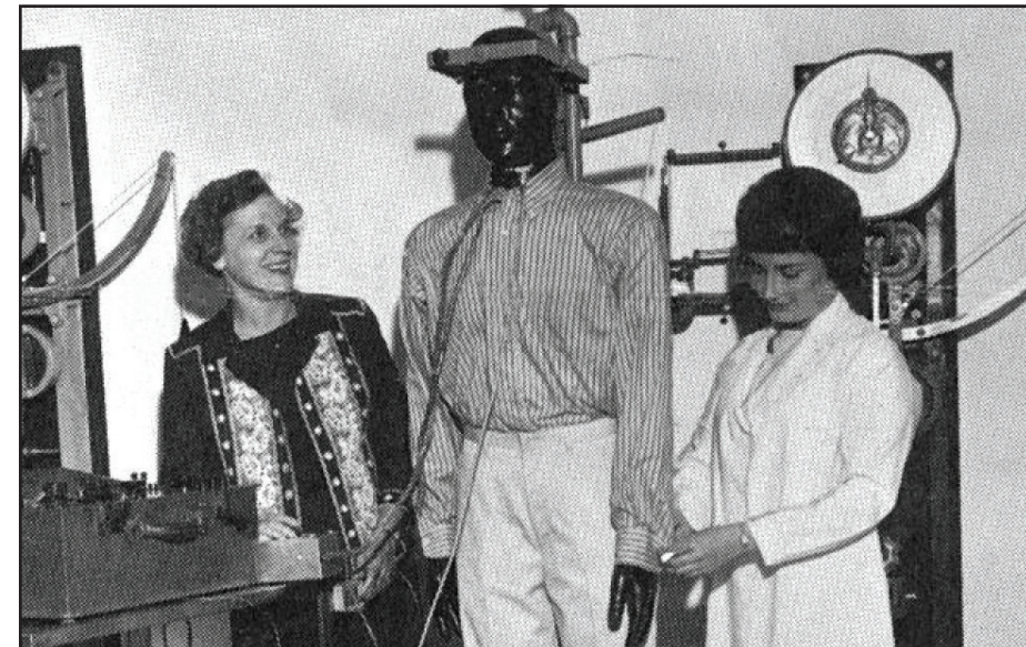
The General Electric Company's life-size copper manikin, a hollow shell in the shape of a human, is on loan to K-State's IER to determine the insulative value of types of clothing.
