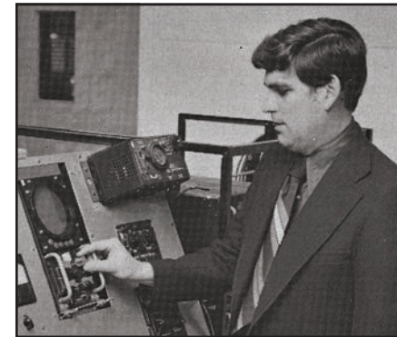
Severe weather within a 100-mile radius of Manhattan will soon be detected on the screen of this radar set designed in the early 1950s for forward surveillance on a Boeing 852. Donald Hummels makes minor repairs on the radar set and recently obtained an FCC license for its operation.
