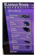
Computer Main – presentation computer hooked up to the system (selected by default). May need to press the keyboard space bar to wake up the computer.
