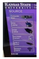
Computer Main – presentation computer hooked up to the system (selected by default). May need to press the keyboard space bar to wake up the computer.
