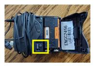
Flip open front of pack, press and hold power button to turn mic on/off.
