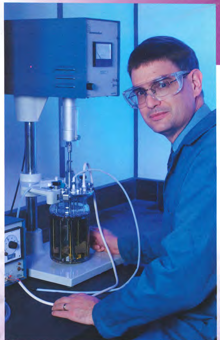
Stevin Gehrke, chemical engineering department head, checks fermenter used for culturing bacteria.
