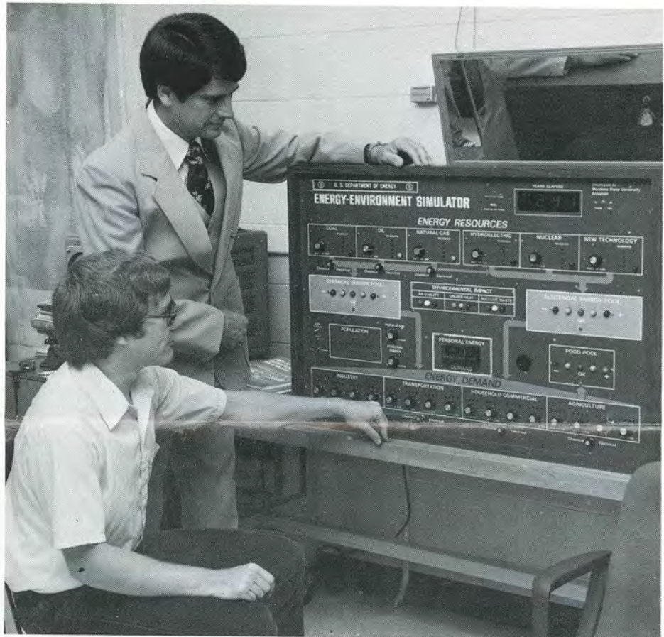
College of Engineering students are using the Energy-Environment Simulator from the College's Center for Energy Studies to teach primary and secondary school students and others how energy supply and demand works. Participants decide which sources of energy they wish to use for various purposes and the computer will then calculate the effect on resources and the environment. At left is Paul Briggs, graduate student in nuclear engineering who directs the program. With him is Richard R. Hayter, director of the Engineering Extension Service, which is primarily concerned with energy conservation.
