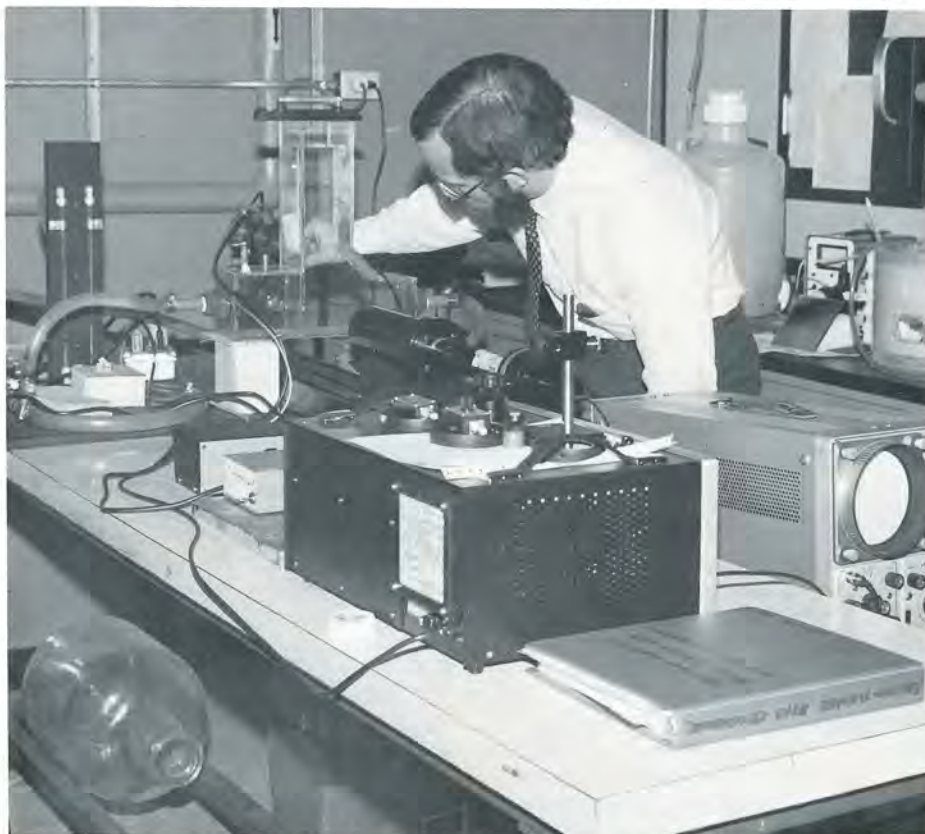
Larry Glasgow, chemical engineering, uses Laser-Doppler velocimeter to study effects of physiochemical environment upon particle size distribution in coagulation.
