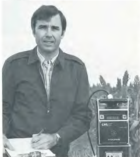
James Koelliker, civil engineering, uses neutron probe as part of a field study to evaluate potential for groundwater recharge in western Kansas.
